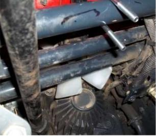
.4 Line up the skid plate in a manner that it line up with the hole on the frame. Check clearances around the skid plate so that there are no points of contact other than the mounting locations
