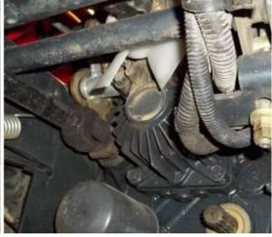
.5 Reinstall the two nylon nuts & washers on the u-Bolt andtightening only, this leave some play that will make it easier to line up the skid plate.
