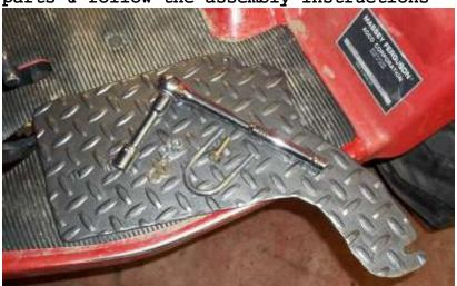
Free up the work place of all disturbance & clutter. Take your time installing it (This can be easily done by one person in 5 to 10 minutes). Have a good look under your tractor, Mower deck will have to be remove to properly install the skid plate.
